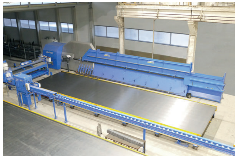
The Pluristar by progress Maschinen & Automation is an automatic stirrup bender, straightener and double-bending machine in one. It was perfectly integrated into the new Ebawe carousel plant.
