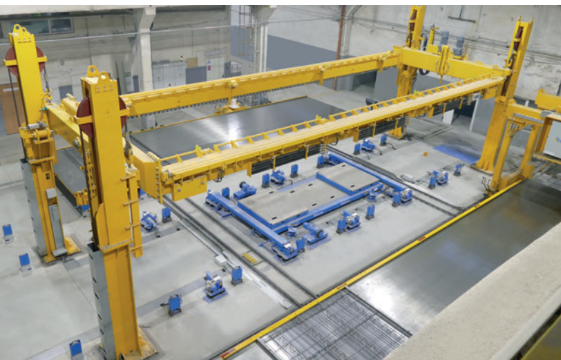
The pallet turning device is the new center piece for the carousel's plant double wall production.
