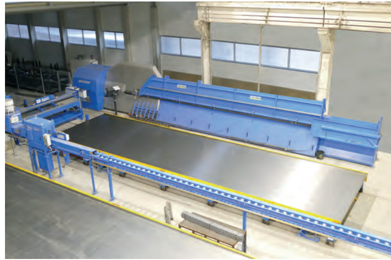
The Pluristar by progress Maschinen & Automation is an automatic stirrup bender, straightener and double-bending machine in one. It was perfectly integrated into the new Ebawe carrousel plant.
