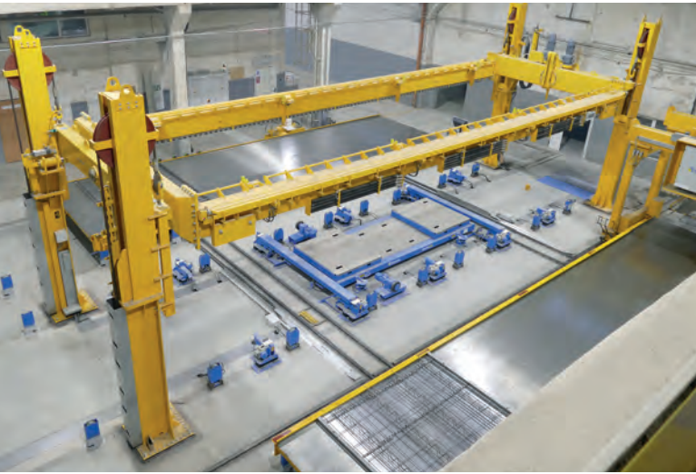
The pallet turning device is the new center piece for the carrousel's plant double wall production.
