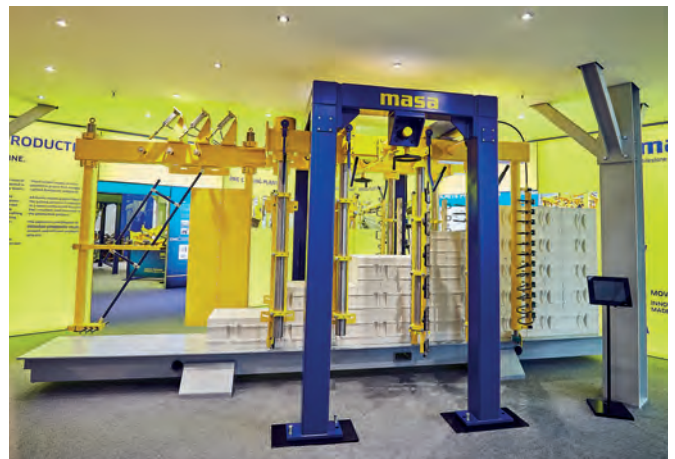
Side cutting and profiling station for AAC products
