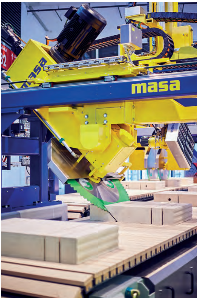
Masa sand-lime brick sawing technology
