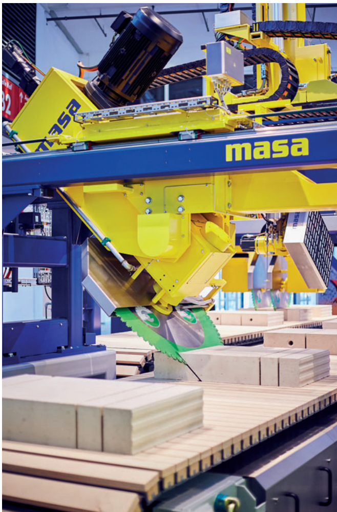
Masa sand-lime brick sawing technology
