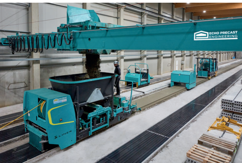
Larco is producing pre-stressed precast concrete elements on four production lines. Heart of the production is the Slipformer S-Liner® from Echo Precast Engineering.
