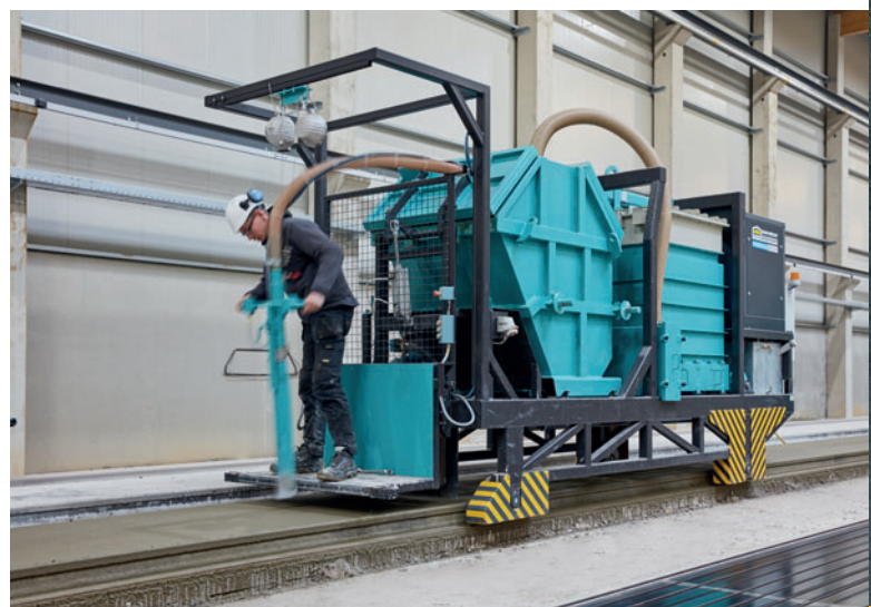
A multi-angle saw, a fresh concrete saw, an automatic plotter, a concrete distributor an absorber and a multifunctional trolley round up the production equipment delivered by Echo Precast.
