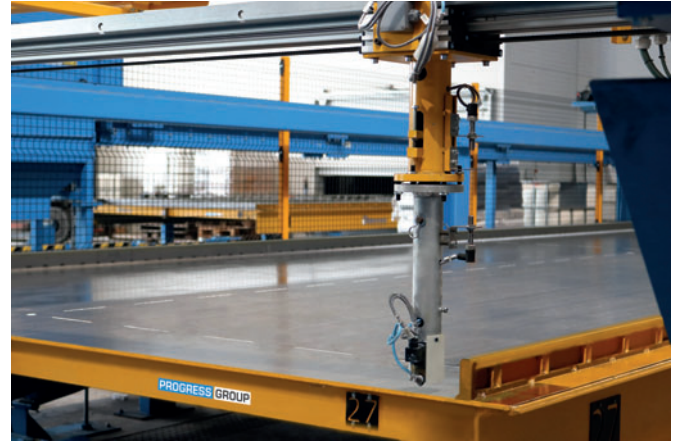
With the help of a plotter, the precast slabs’ contours as well as electricity boxes or other elements, are plotted on the pallet in order to make the manual shuttering process precise and time saving.
