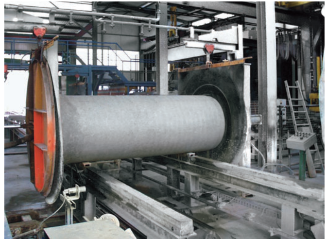
Vacuum pipe testing device for the leak test
