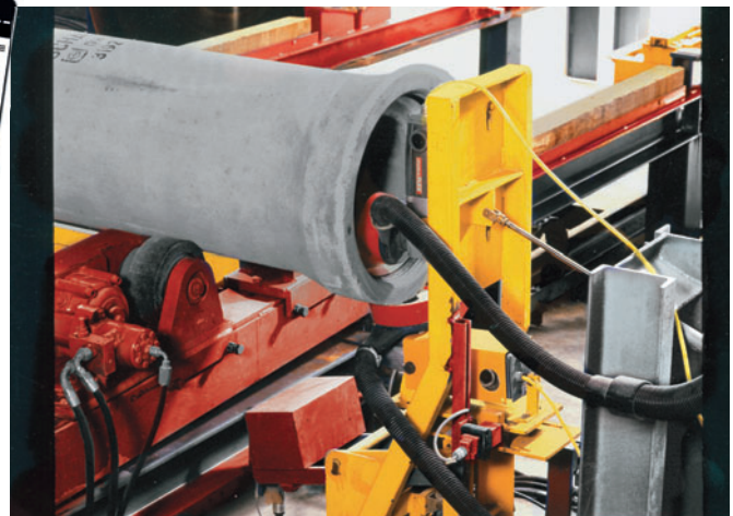
Deburring station for processing internal and external bell diameters and the spigots of concrete pipes
