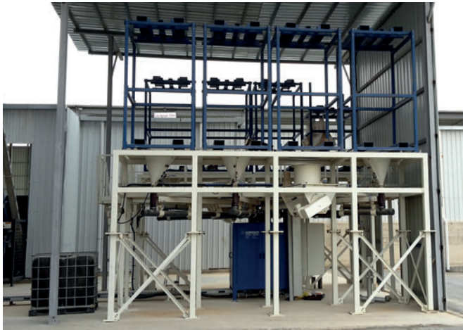
)) The 8-colour dosing system FLEX 70-1 from Würschum GmbH.
