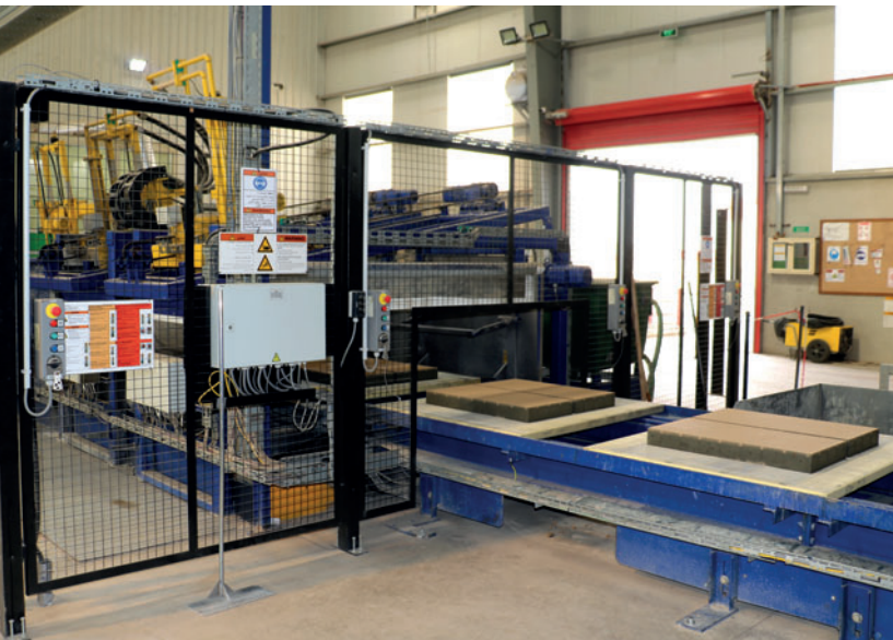
Masa paver washing unit with 3 stations.
