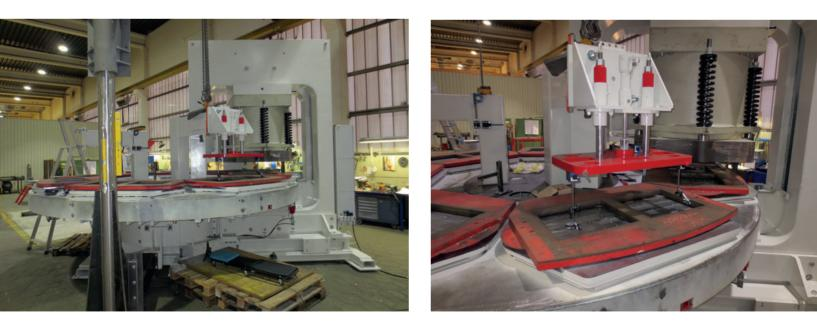
Optimised facing concrete distribution and compaction, automatic fine adjustment of the facing concrete distributor and ejector and a decoupled turntable-press system - those are the new features of the hermetic press for the manufacture of concrete slabs that SR Schindler will be presenting at the bauma 2019.
