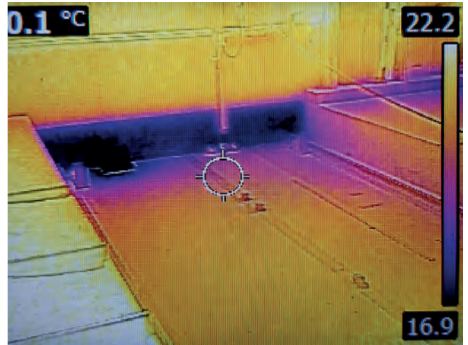
Dark purple areas at the chamber outside perimeter walls lighten slightly as the floor becomes warmer further away from the walls. The high amount of purple throughout the picture indicates poor air circulation.
