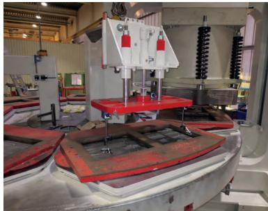
Optimised facing concrete distribution and compaction, automatic fine adjustment of the facing concrete distributor and ejector and a decoupled turntable-press system - those are the new features of the hermetic press for the manufacture of concrete slabs that SR Schindler will be presenting at the bauma 2019.
