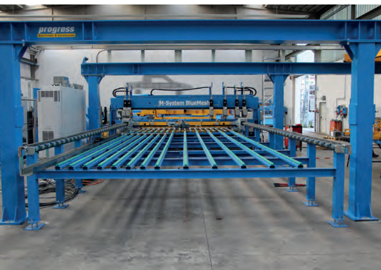
Sansiri integrated a new BlueMesh M-System, a mesh welding machine from progress Maschinen & Automation into their carousel plant for precast concrete elements.
