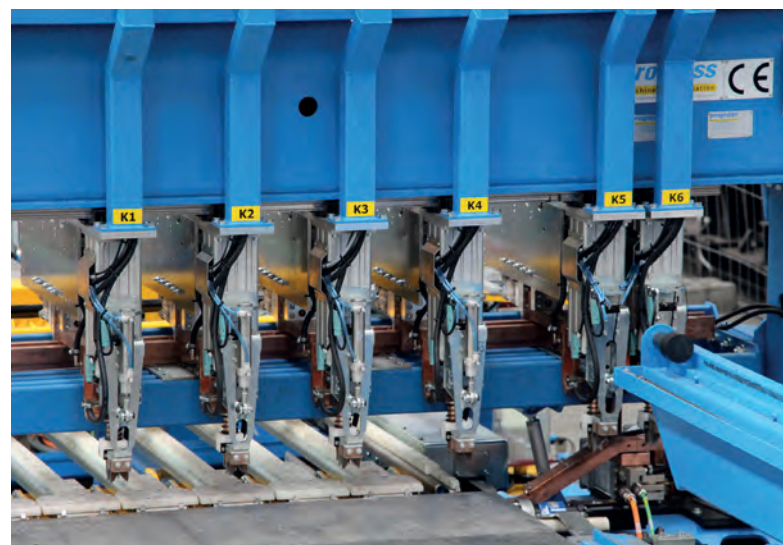
The welding machine is designed as a flexible production plant for reinforcement mesh directly from coil according to individual specifications.
