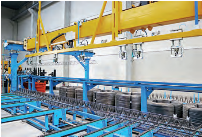
The Progress lattice girder welding and handling machines of the VGA Versa series represent the best in flexible, just-in-time lattice girder production.
