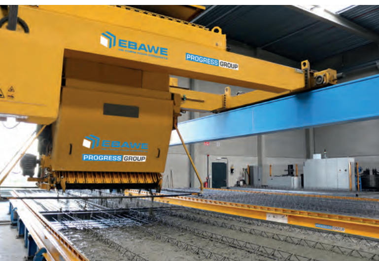
The automatic concrete spreader ensures an even and optimized distribution of the concrete into the moulds.
