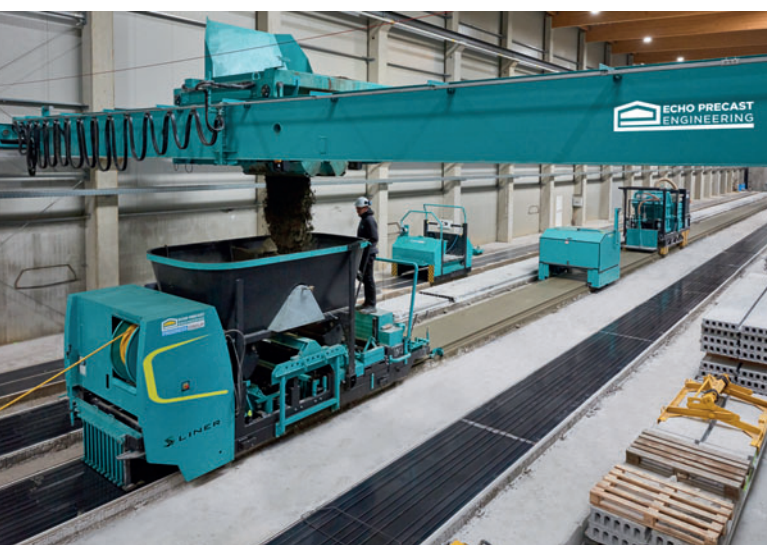
Larco is producing pre-stressed precast concrete elements on four production lines. Heart of the production is the Slipformer S-Liner® from Echo Precast Engineering.
