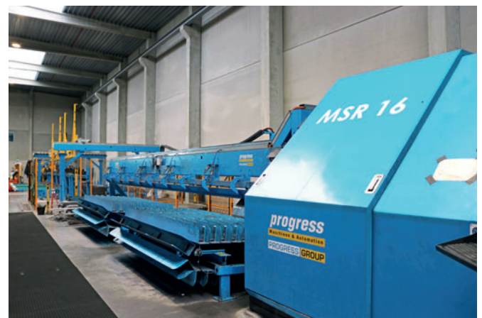
The Progress MSR 16 straightening and bending machine works off coil and optimizes the flow of production. Low storage costs and easier material handling ensure a cost-effective production.
