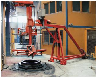
Fully automatic base pallet insertion equipment
