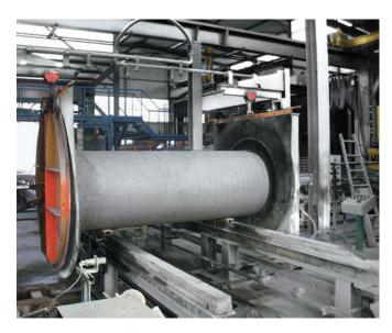
Vacuum pipe testing device for the leak test
