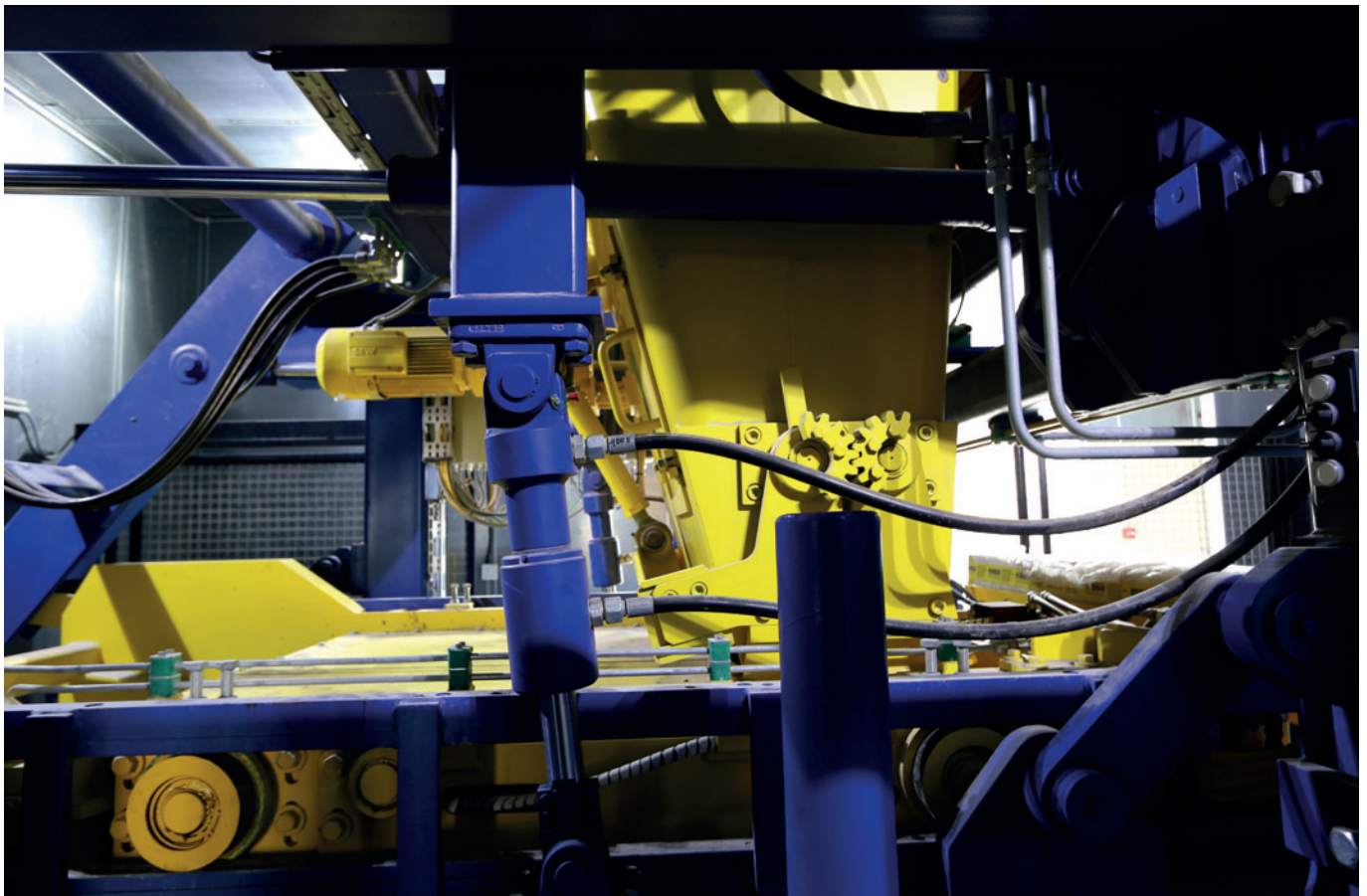
View into the Masa XL - The face mix concrete is dosed directly into the filling box via a silo flap.
