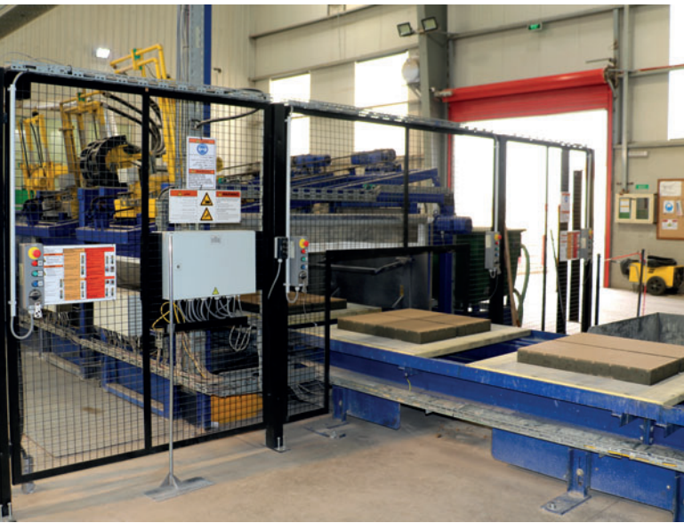
Masa paver washing unit with 3 stations.
