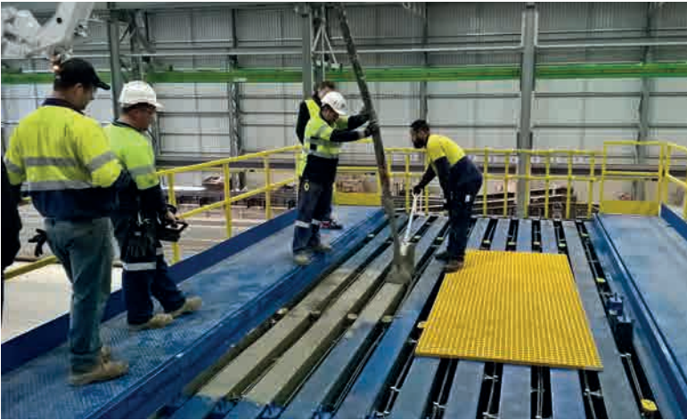
Battery moulds for concrete precast wall elements offer a high productivity in limited space. BGC produces up to 20 wall elements per cycle.
