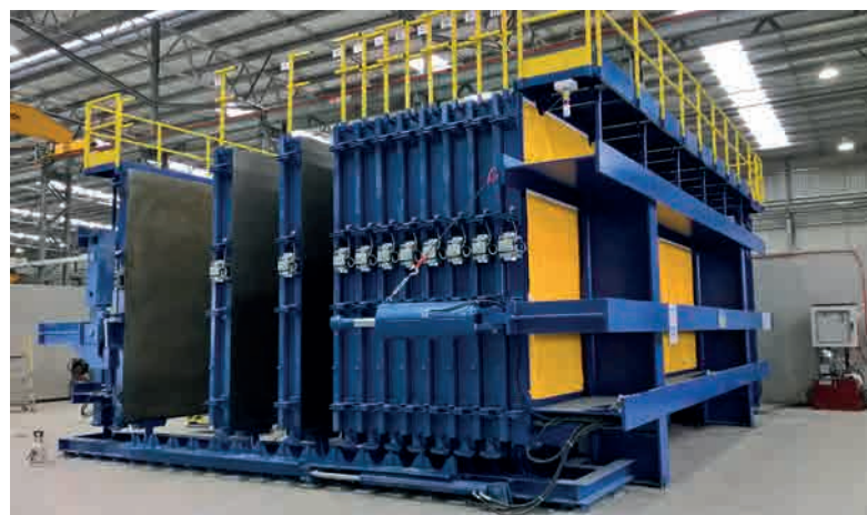
The battery mould from tecnom was installed in 2017 at BGC, who is the first company in Western Australia to use such an equipment.
