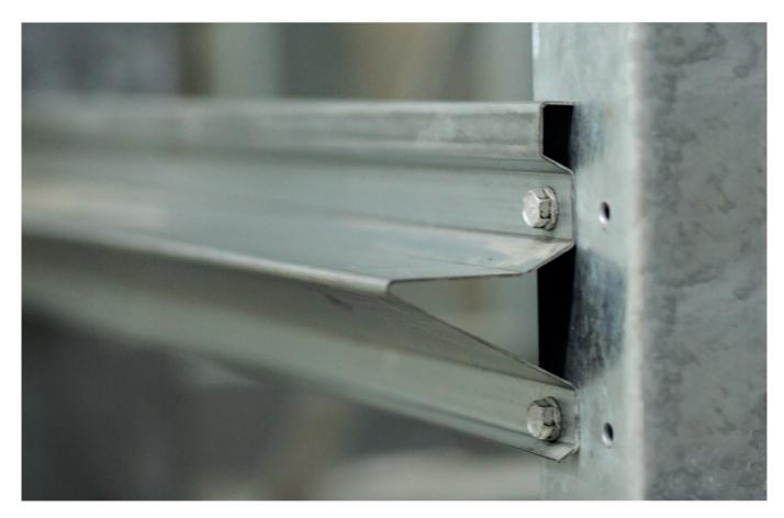
Design of the Kraft Curing Rack shelf: the connection is secured against failure, the profile is highly torque resistant and the integrated board guide provides for secure alignment of production boards in all areas.
