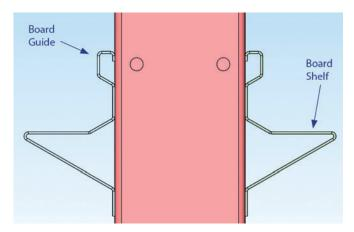
Drawing of the Kraft Shelf Profile. Board shelf and board guide are connected in one piece. Production boards are precisely and securely guided over the full depth of the rack.
