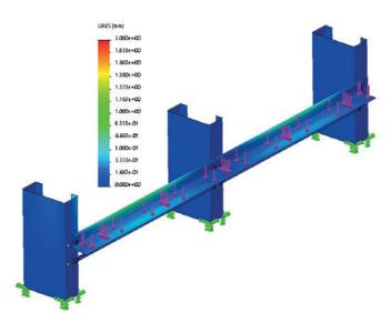
The Kraft Rack shelf profile was designed to withstand stress and torque. Computer analysis (Finite Elements Analysis - stress comparison) shows that profile is capable of absorbing high loads (simulation shows a deformation of less than 1mm at a load of 750kg per board shelf).
