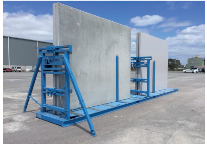
Wall elements produced with battery moulds from tecocom excellent quality and finish of the elements. Both the two wall faces have a smooth finishing. (Credits: BGC)
