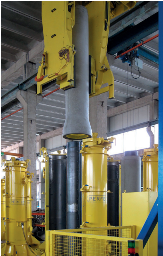
Using Schlüsselbauer's Perfect Forming Technology makes high quality concrete pipe production quite comfortable: The cured product can be easily stripped from the mould independent from degree of automation.
