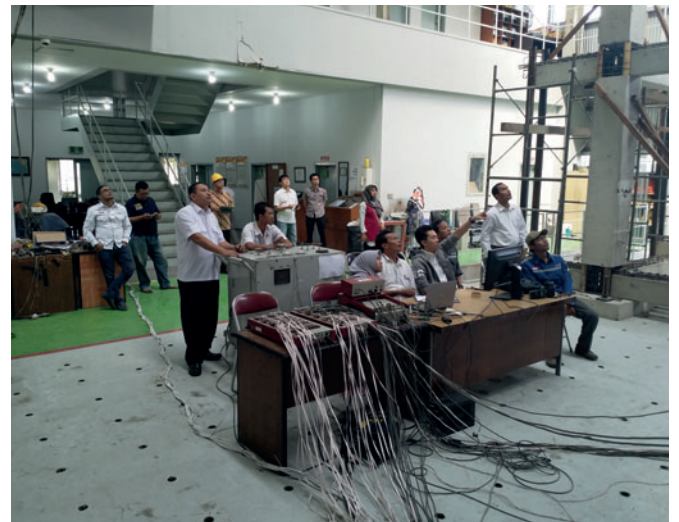
A test building made of precast concrete elements was subjected to a seismic test at a building materials testing body.
