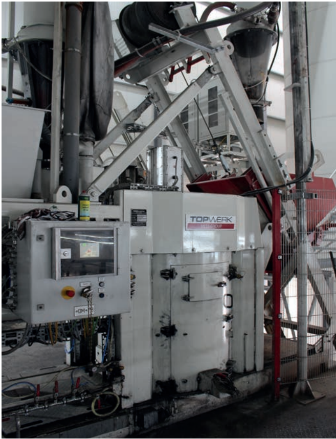
The Hess SM 400 mixer produces the facing concrete.
