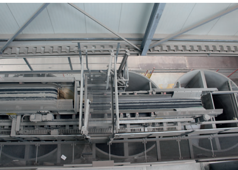
Here too, a distribution belt ensures the correct feeding of the individual silos.
