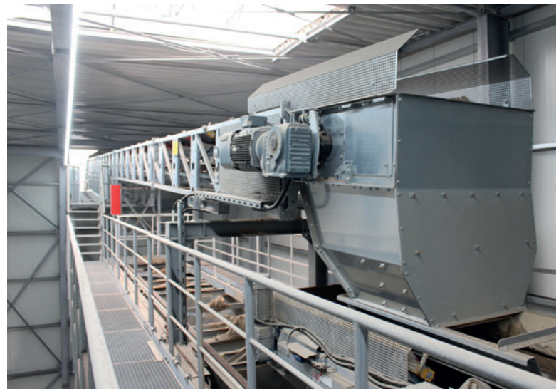
The core concrete aggregates are transported by a new conveyor belt from the adjacent original hall.
