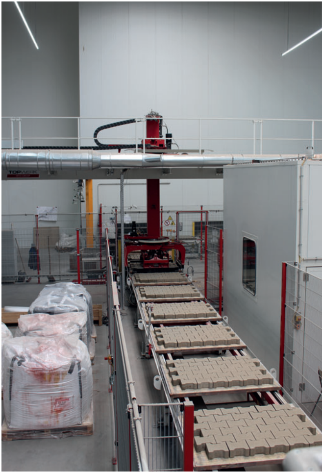
The first cuber is located behind the bypass. This either releases the stones or supplies the refinement machine from SR-Schindler with concrete products.
