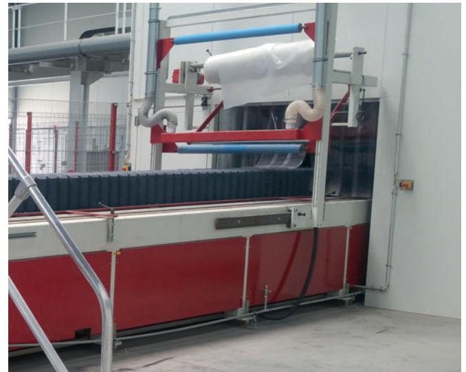
A Mega 6000 Duo aging machine from SR-Schindler was integrated as a bypass system on the dry side for the refinement of the concrete products.
