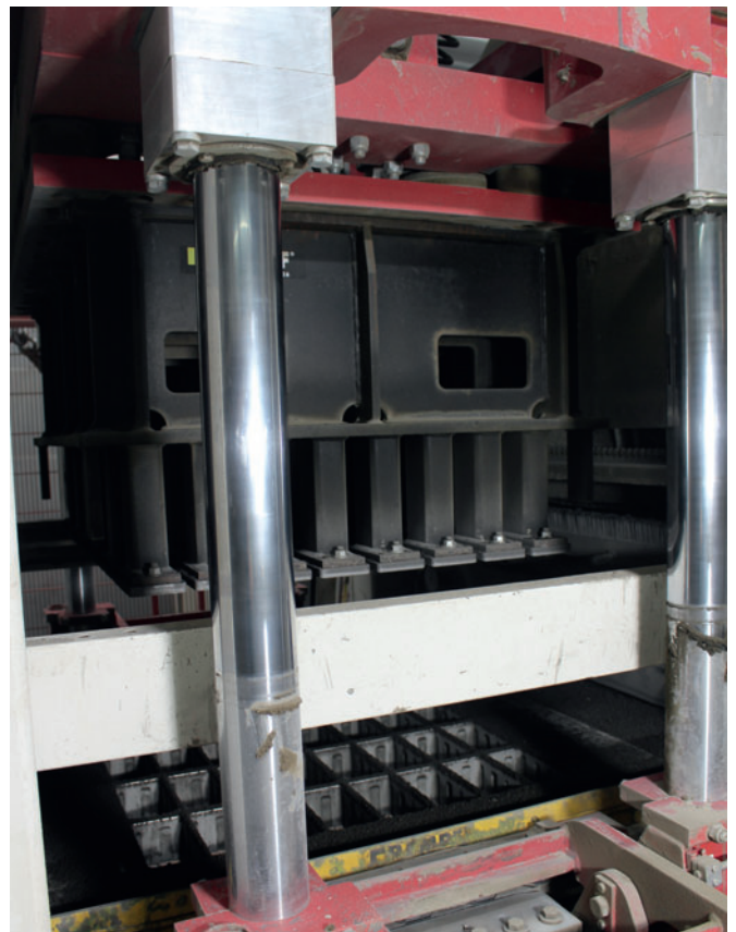
Hess Multimat RH 1500-3 block making machine
