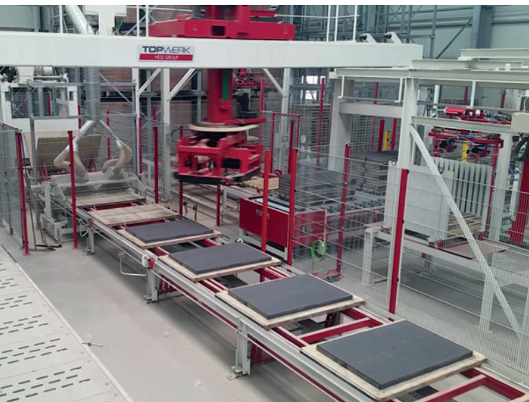
The second cuber has access to both the finishing line and the "normal" line.
