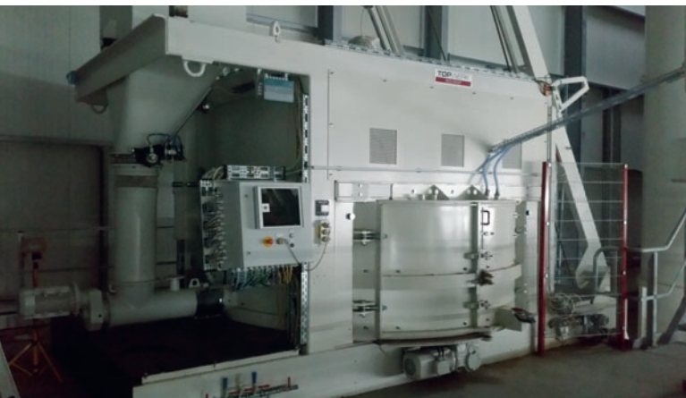
Hess SM 3375 core concrete mixer
