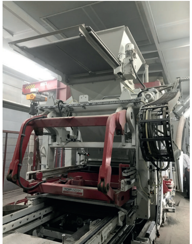
Hess Multimat RH 1500-3 block making machine
