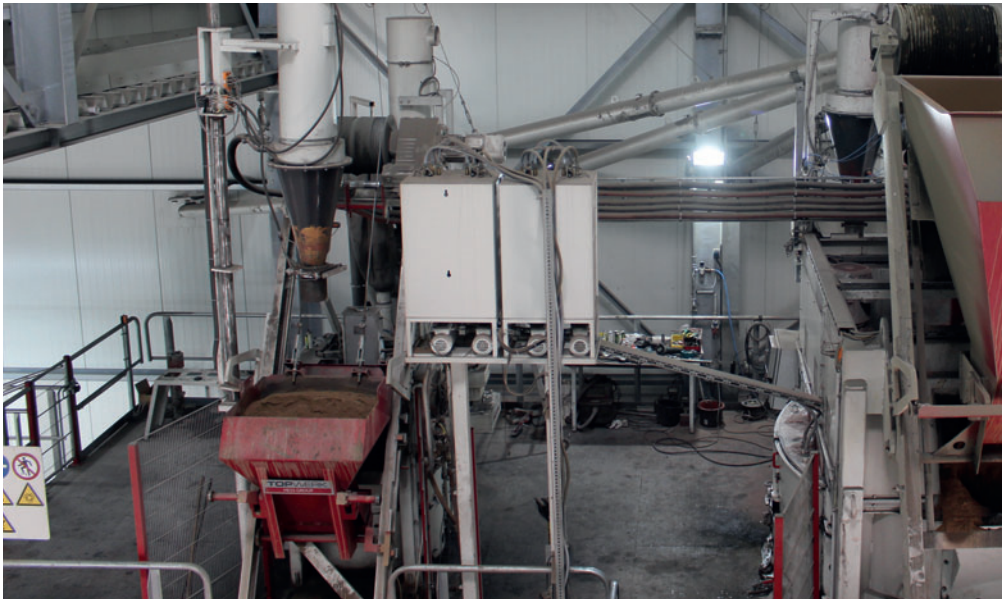
Two compulsory mixers from the Hess SM series were installed on a mixer platform for the production of the concrete.
