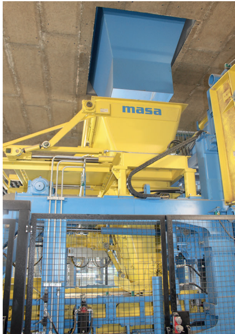
Core and facing silos are equipped with weighing cells
