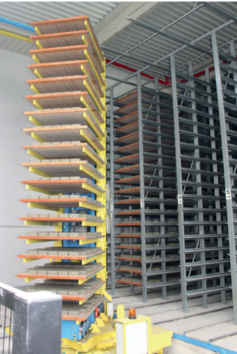
Finger car with a load capacity of 20 tonnes
