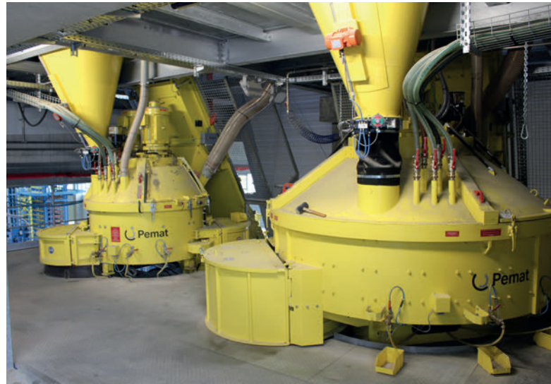
High-performance Pemat planetary mixers for continuous concrete production
