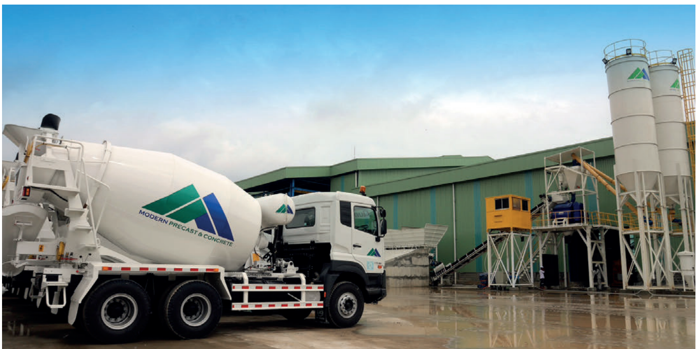
The new mixing plant has a capacity of 500 m 3 per shift. Modern Precast currently operates a fleet of six truck mixers, each with a capacity of 7 m 3 .
