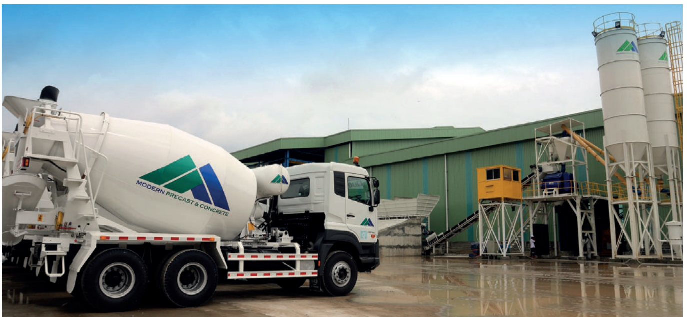
The new mixing plant has a capacity of 500 m 3 per shift. Modern Precast currently operates a fleet of six truck mixers, each with a capacity of 7 m 3 .
