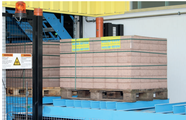
The packets are transported to the outside by trolley car
