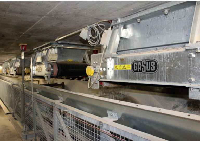
With a capacity of 3,000 kg/min the individual aggregates are weighed additively by dosing belts onto a weighbelt
