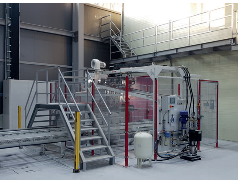
A double washout unit is installed in the transport system on the wet side.
