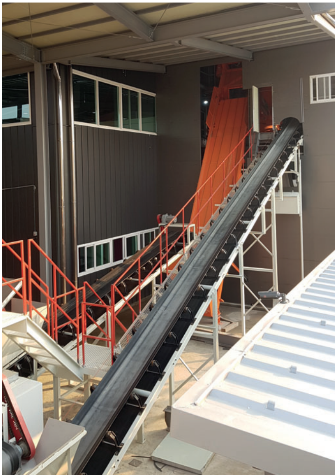
A dosing belt under the bunkers weighs the aggregates for the core concrete and fills them into the lifting bucket.
