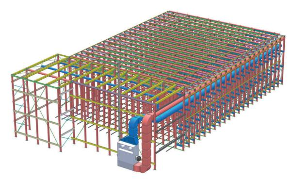
Rack design with fully integrated Quadrix curing system. The insulated chamber provides storage for concrete products on 6,000 production boards and more to harden.
