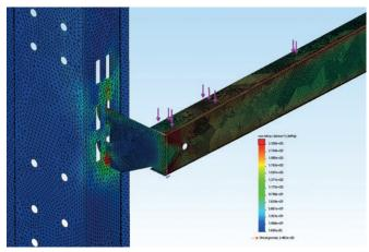
The FEM calculation indicates the weak points in a traditional rack shelf. Using the identical load as previous, this unit is substantially weaker and more prone to deformation and failure.
