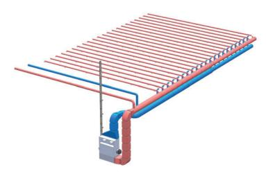
Installing the Quadrix curing system is made easier and less expensive thanks to less distribution duct and fewer different cross sections
