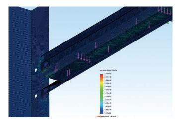
Shelves in the newly developed Kraft design. Its appreciably greater loading capacity is clearly shown up in the FEM analysis. The shelf's profile and height generate the high load capacity. The integrated guide rails over each passage's entire length make it impossible for the production boards to shift out of line – something that can otherwise cause irreparable damage to the rack columns.
