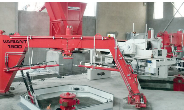
Variant 2500/1500 concrete pipe machine during installation
