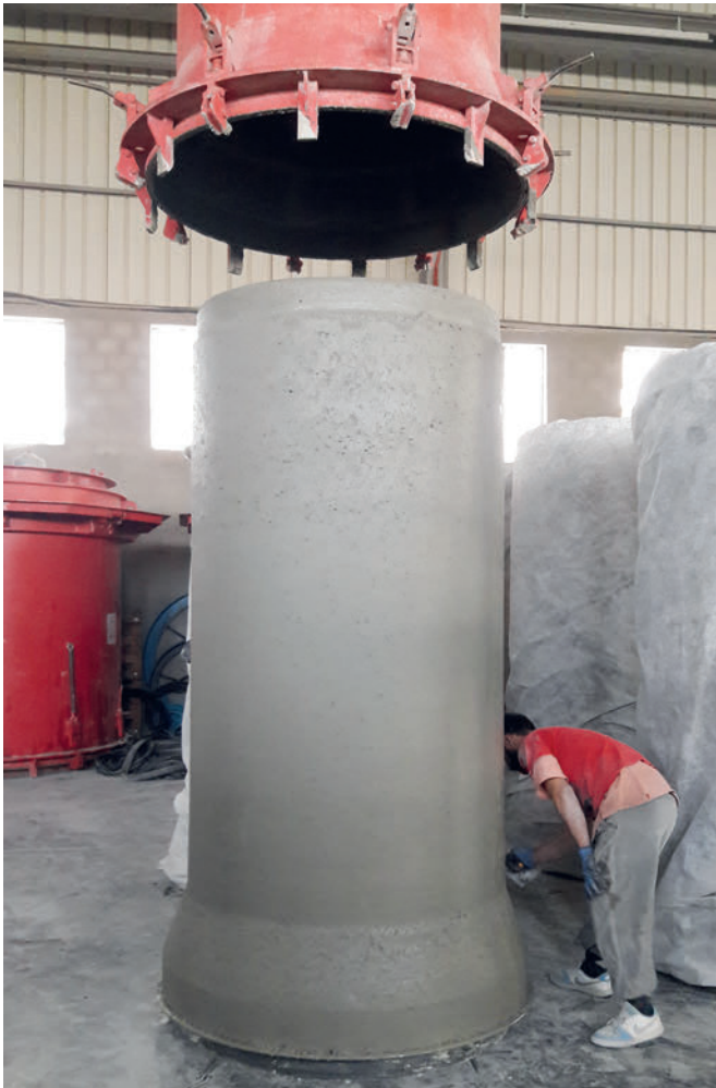
Concrete pipe after demoulding
