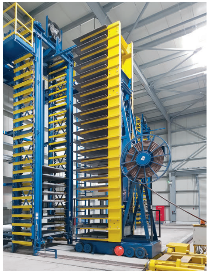
View to the finger car in the curing area.
