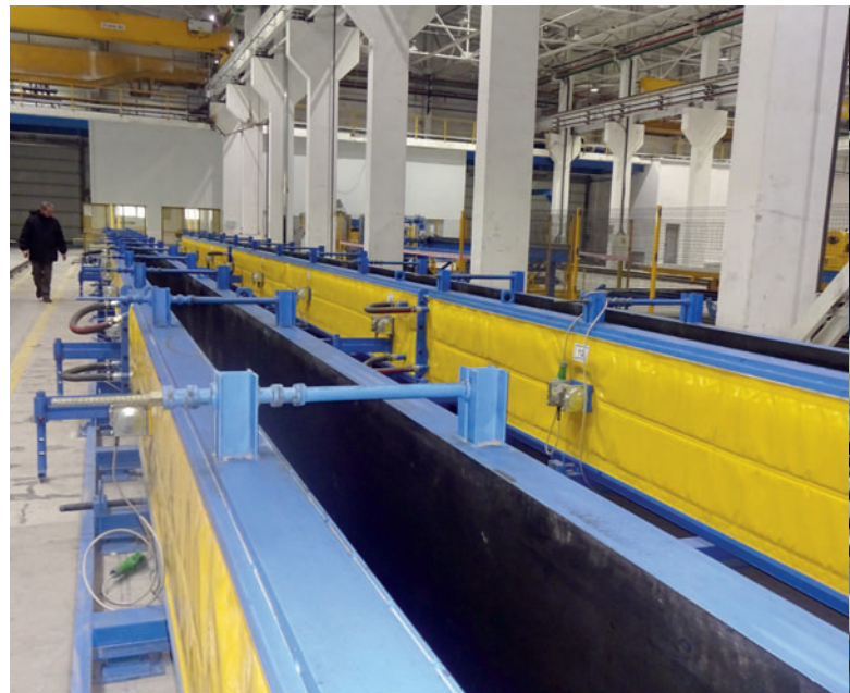
The shuttering specialist Tecnomac supplied both battery moulds and shuttering for the production of columns and beams.
