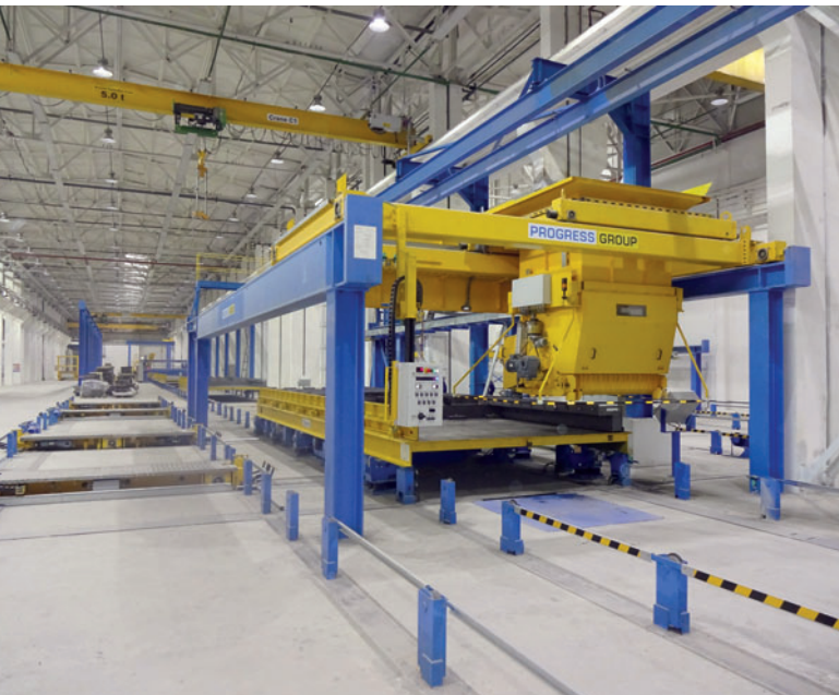
A total of 41 production pallets are available to Erel in the pallet circulation plant from Ebawe Anlagentechnik.
