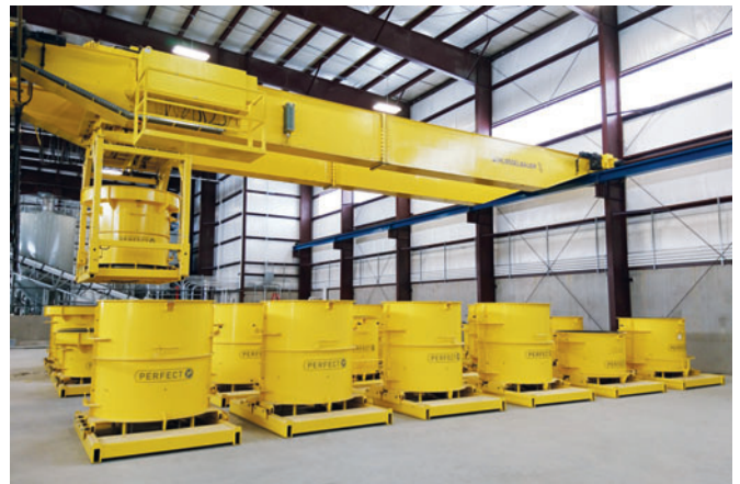
Filled moulds are handled using robotic cranes, which means there are no cycle time losses caused by manual handling, and forklifts are not constantly moving around the factory floor
