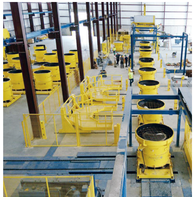
The Perfect Forming Technology production system in CP&P's plant in Ashland provides the most efficient way of producing manhole bases nationwide
