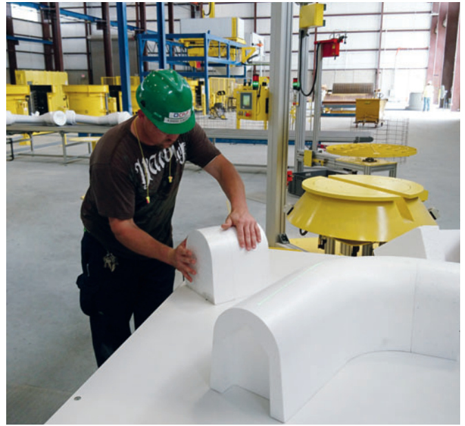
The prefabricated EPS parts are cut with hot wire saws and can be easily combined into channels of the required shape
