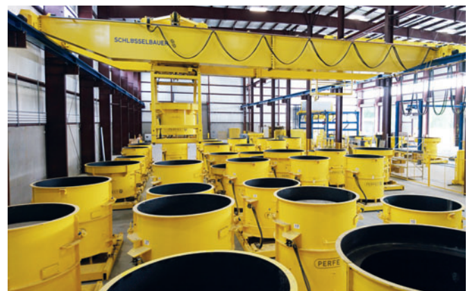
Easy-to-operate moulds provide the capacity and flexibility required to manufacture manhole bases
