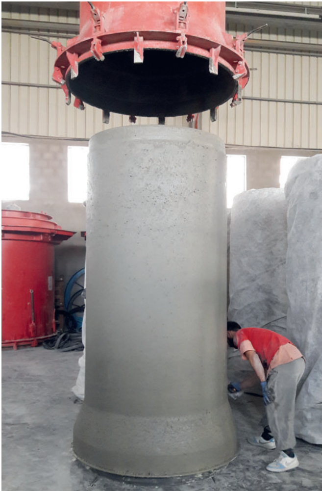
Concrete pipe after demoulding
