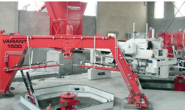
Variant 2500/1500 concrete pipe machine during installation
