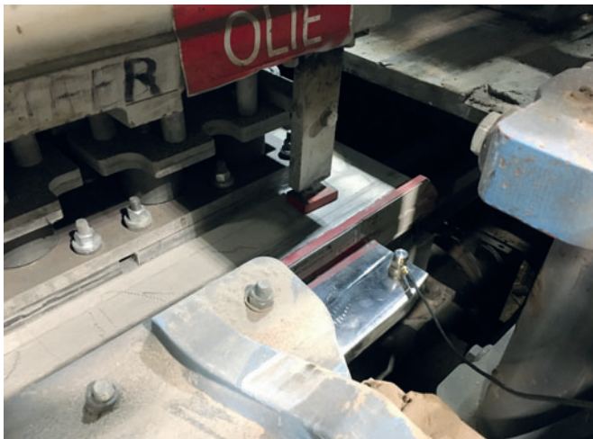
Figure 3: Vibration measurement on the concrete block mould
