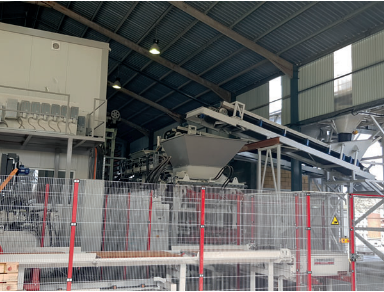
Feeding the RH1500 with production boards and concrete
