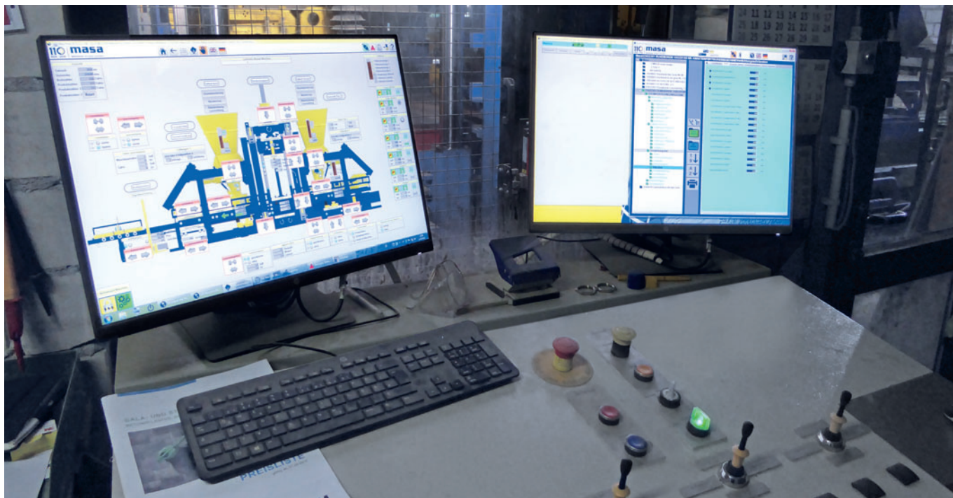
The modular Masa system control software for uniform operation and visualization of the components has been supplemented by a data transfer interface.
