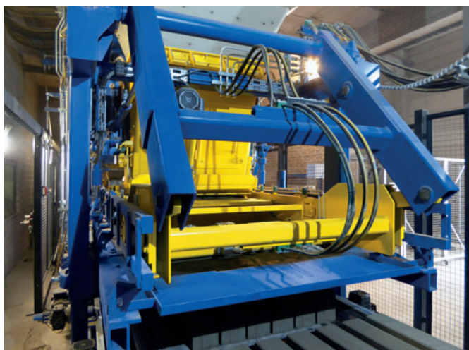
..., since an amplitude-controlled drive of the vibrators is used
