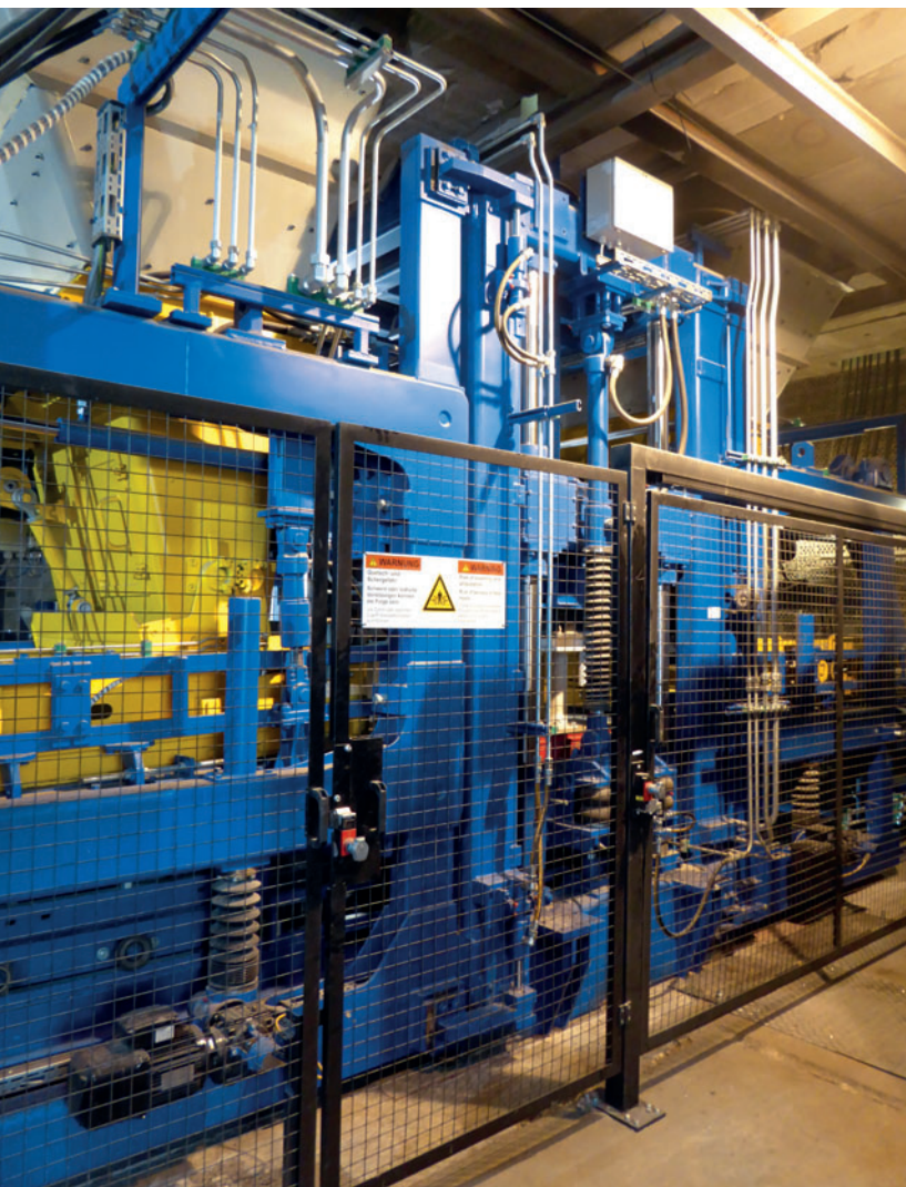
During the production cycle, the vibration force can be adjusted independently from the rotational speed, ...
