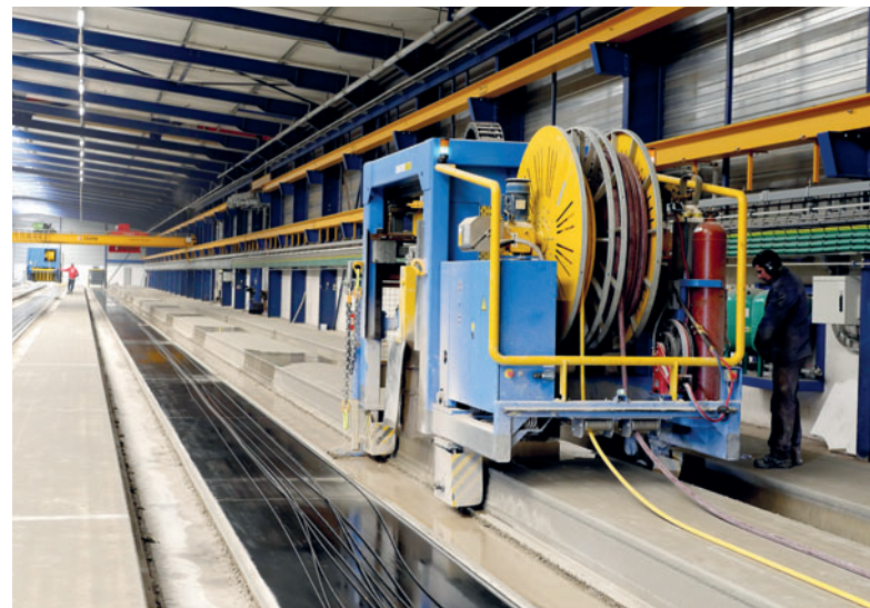
The automated Multi Angle Saw for cutting the Hollow Core slabs at the desired length.
