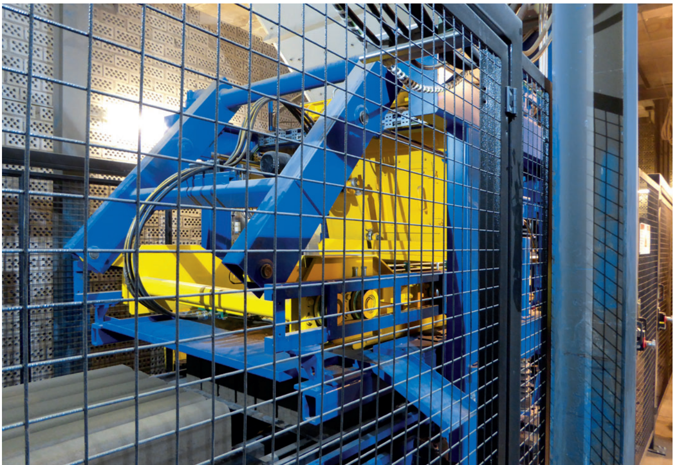
Masa integrated the Masa concrete block making machine L 9.1 into an existing plant in Elxleben, Germany.
