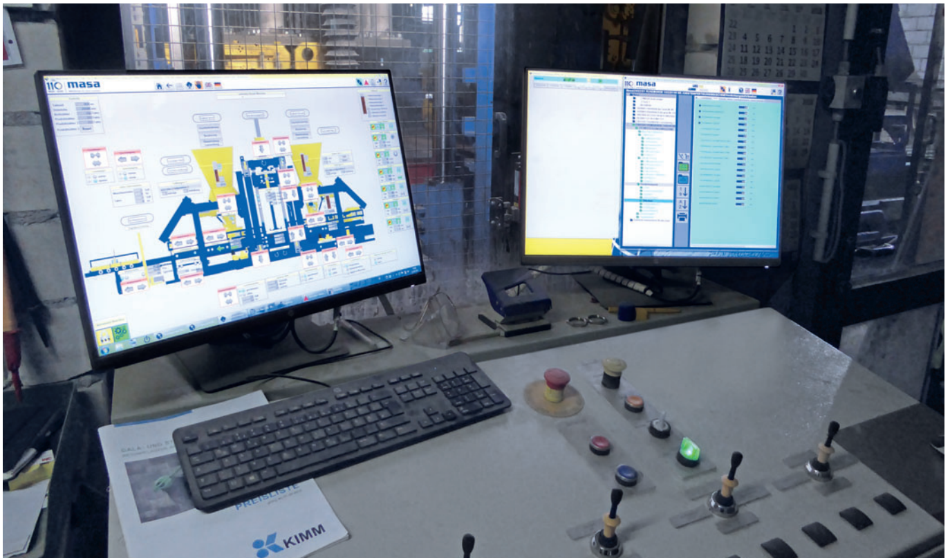
The modular Masa system control software for uniform operation and visualization of the components has been supplemented by a data transfer interface.
