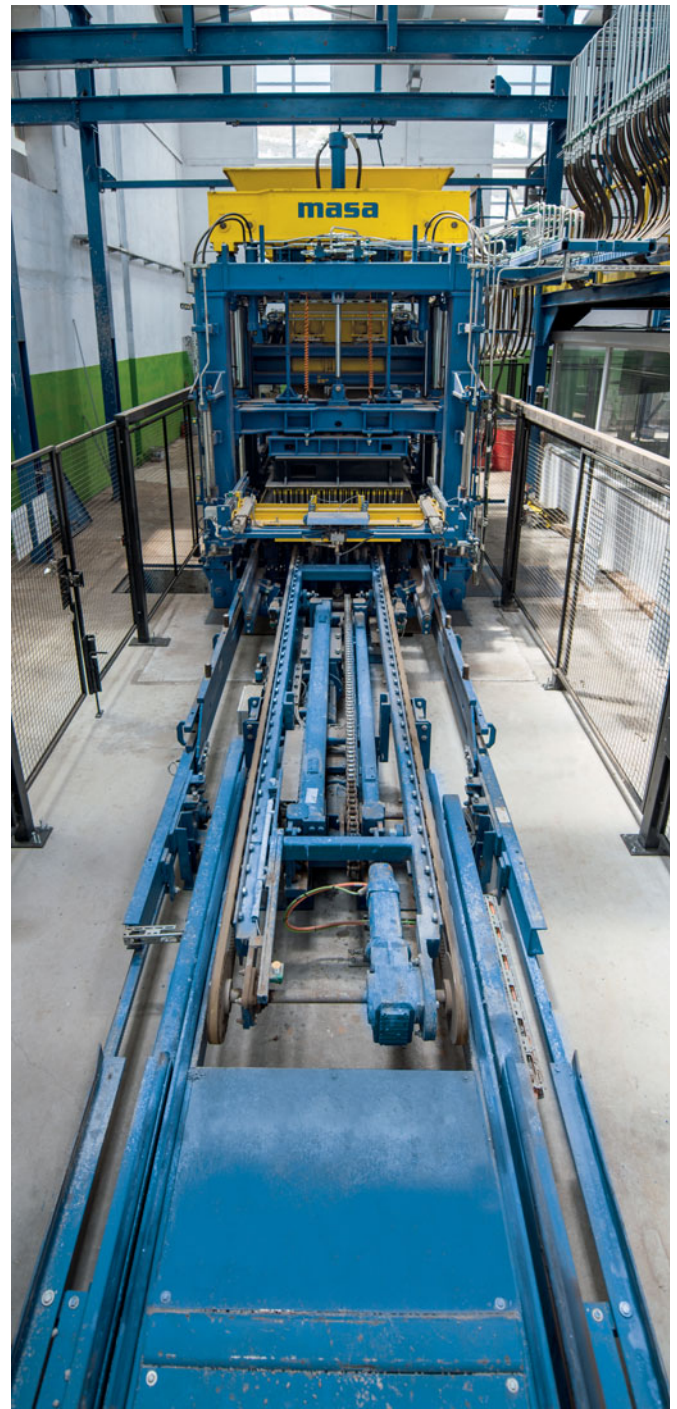
Fig. 1: The heart of every concrete block making plant: The amplitude-controlled Masa XL 9.2 (main mix concrete machine) is equipped with an additional package
