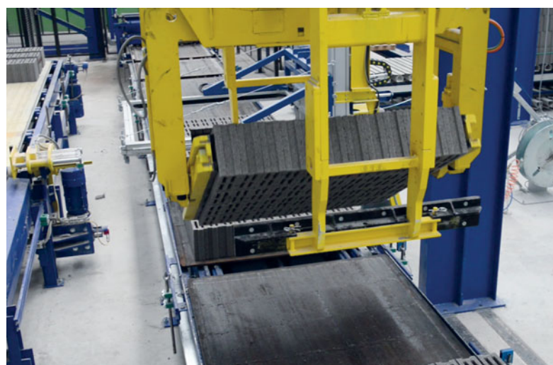
Fig. 4: The clamping basket of the layer shifter is equipped with a vertical turning gear.
