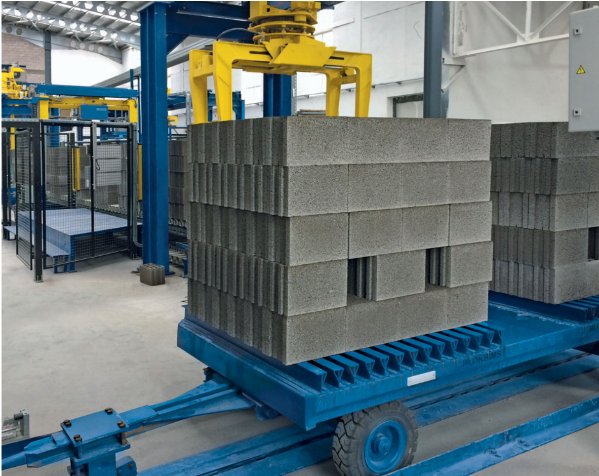
Fig. 6: A cube shifter sets the cubes on transport vehicles, which are coupled to an underfloor conveying system.
