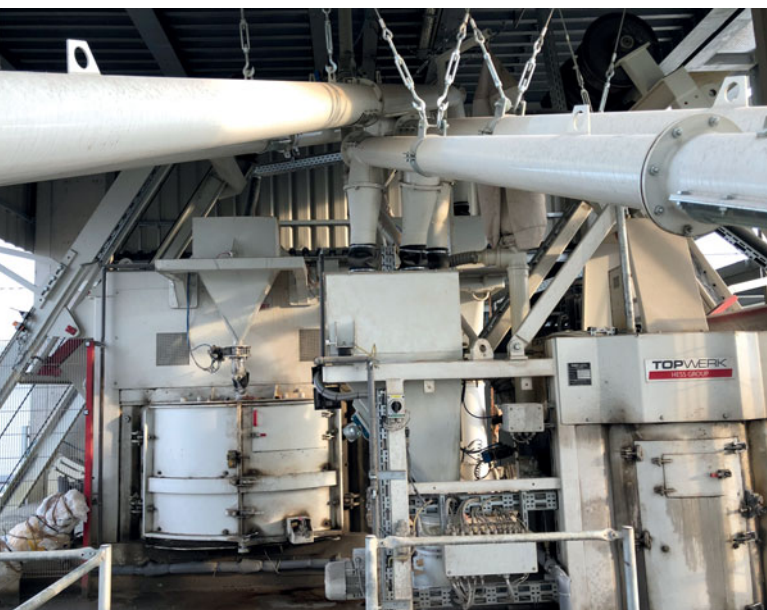
For the manufacture of concrete a Hess SM 2250 concrete mixer was installed for the core concrete and a Hess SM 400 concrete mixer for the facing concrete.
