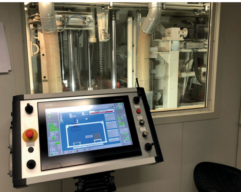
The controller of the RH 1500 MVA is equipped with a large touch screen.
