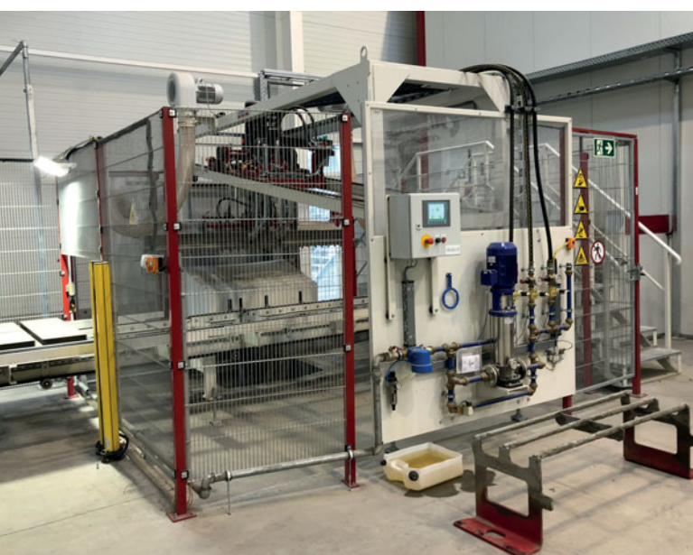
The products can be refined while still on the wet side with a newly developed washing unit from the Hess Group.
