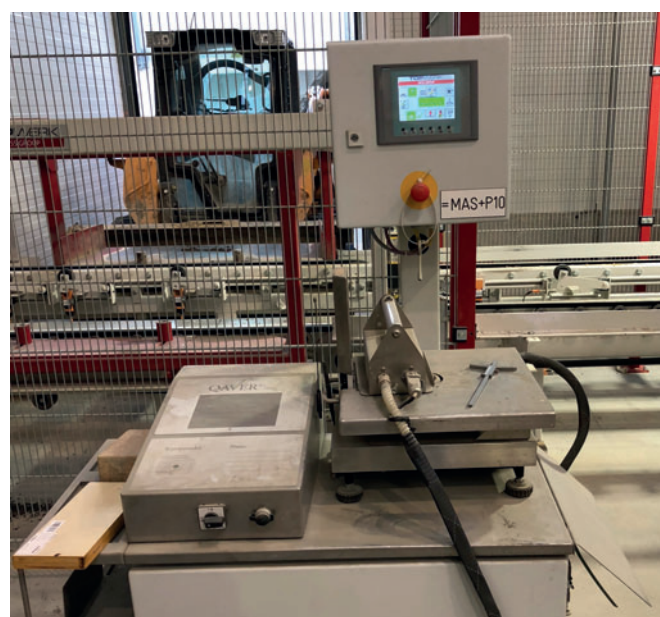
The quality of the products manufactured can be determined directly with the concrete testing device from Qavertec.
