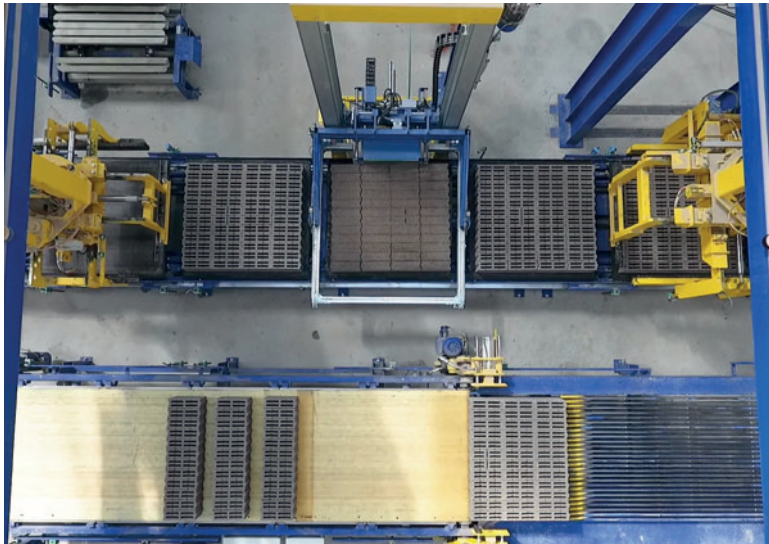
Fig. 5: Principle of the "void layers": A take over and pushing table, a hold-down device and a separating table create the "gaps".
