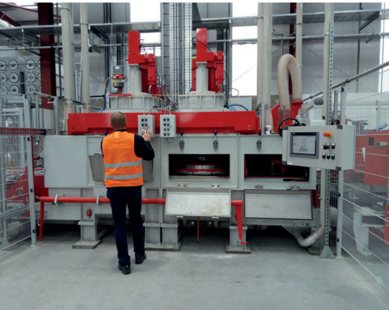
The calibrating machine with two stations operates in dry mode
