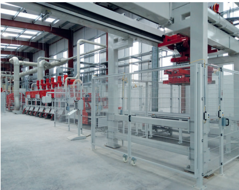
Layer transfer device with electrical 4-sided clamp
