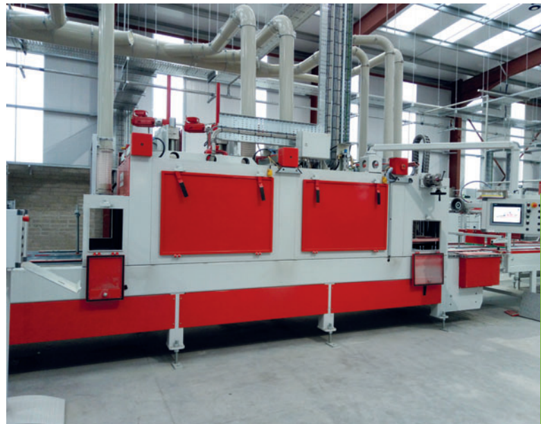
In the curling machine, too, the lateral guides are adjustable electrically to different product widths in inching operation.
