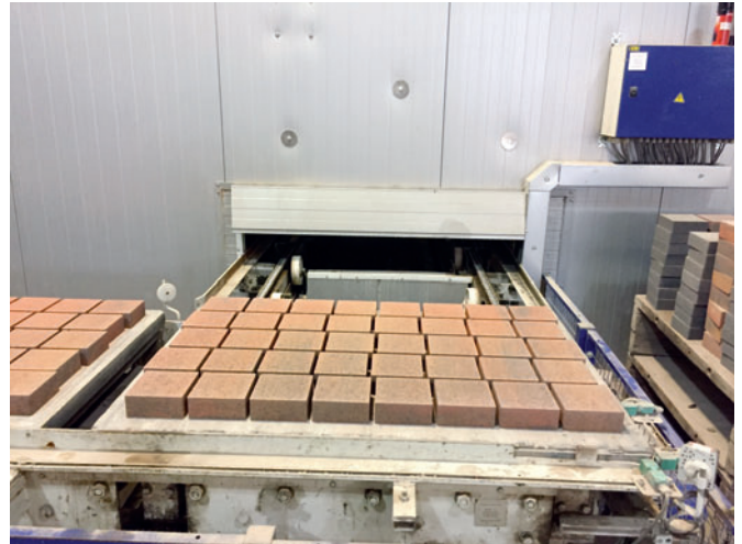
Hardened brindled multi-color pavers leaving the curing chamber after 18 hours.
