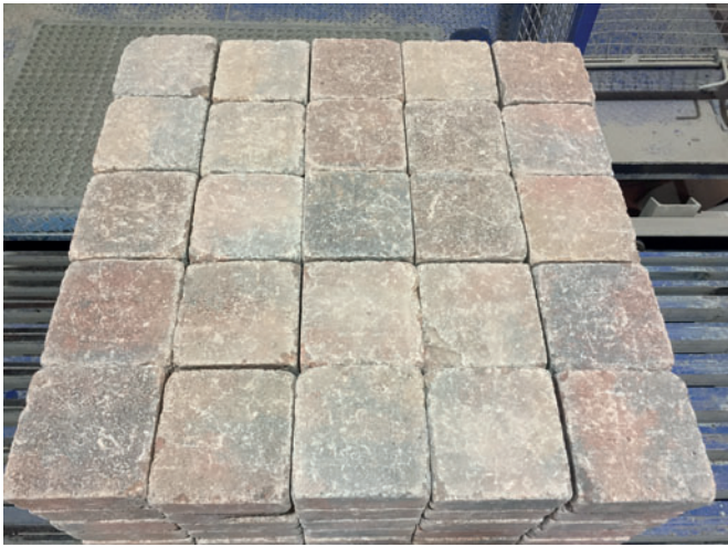
Tumbled paver surface ready for packaging.
