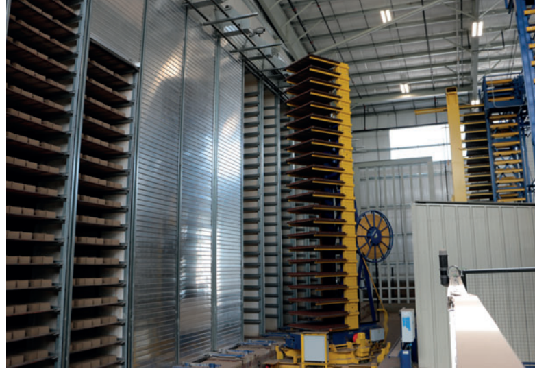
The rotating finger car loading the individual door kilns
