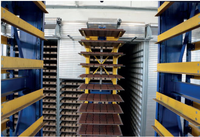
The finger car moving freshly-produced products to the curing racks
