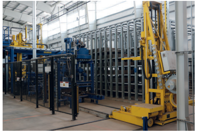
The 2016 capacity ballet buffer with finger car transport system
