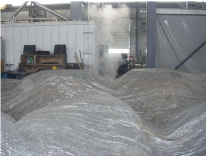
Vapor cured precast concrete elements under a curing tarp.
