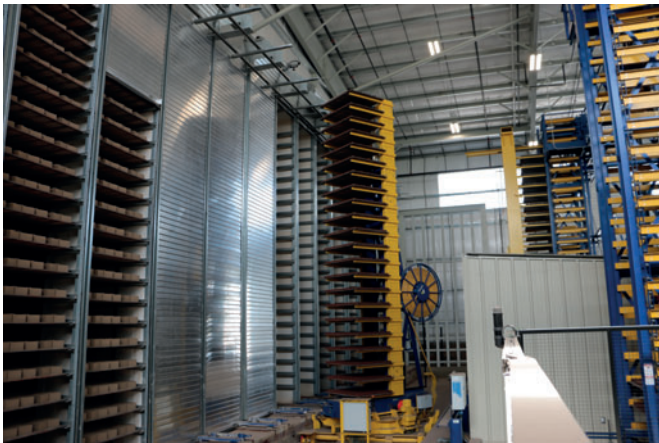
The rotating finger car loading the individual door kilns
