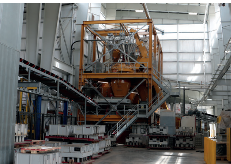
A central raised platform holds the entire mixer operation for both plants
