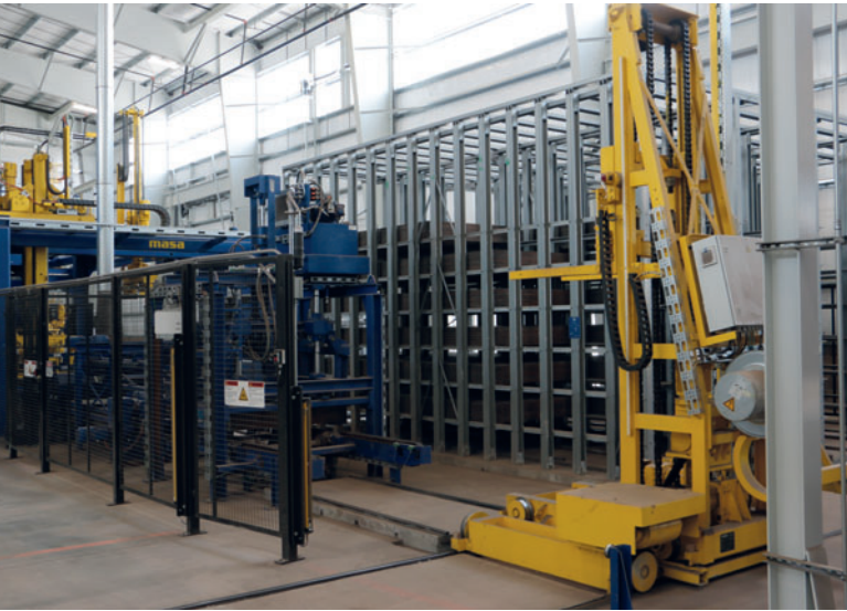
The 2016 capacity ballet buffer with finger car transport system
