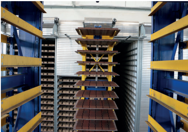
The finger car moving freshly-produced products to the curing racks
